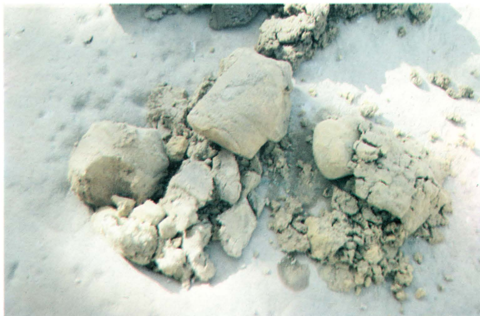
B.— Representative subsurface soils core. [Cliché Hany Helal].
