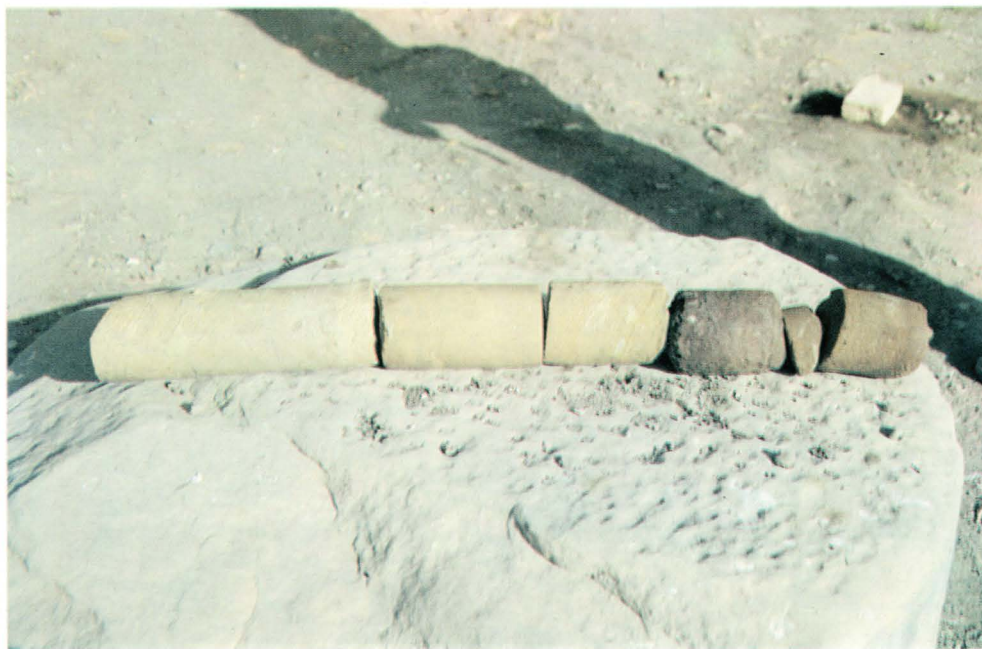
A.— Representative foundation core. [Cliché Hany Helal].
